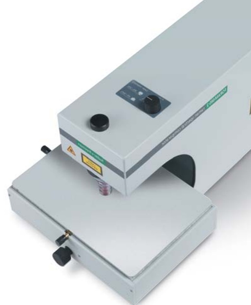
The Foram has a precision X-Y translation stage for accurate laser alignment.
